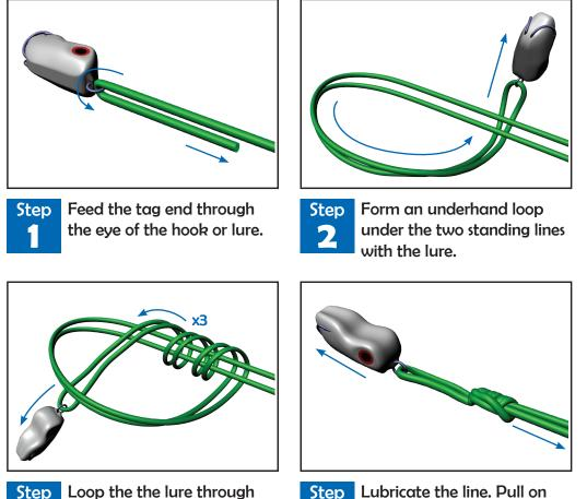
Lubricate the line. Pull on the lure and the line to tighten the knot.
